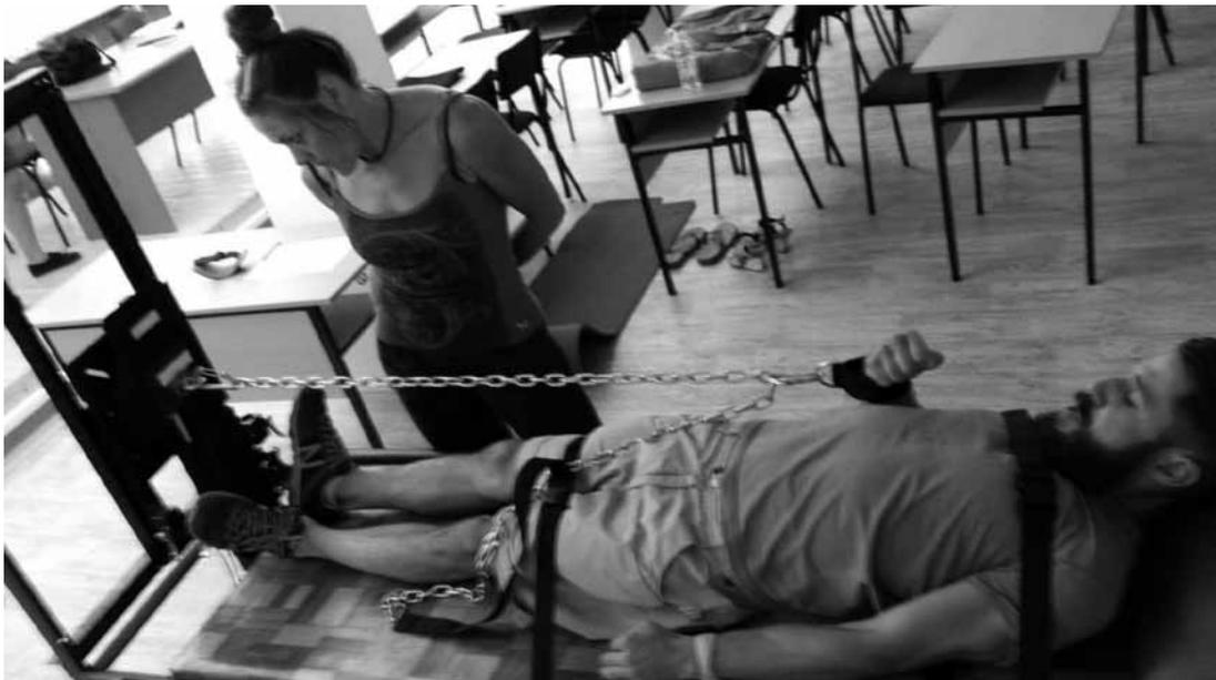
**Figure 1.** *Body and arm position during dynamometry using 3DSAC*
